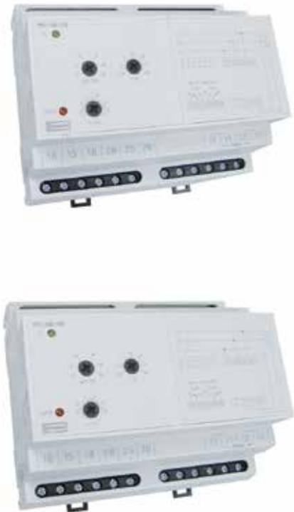
The Reverse Power protector trip relay monitors a single- or three-phase supply for reverse power and trips a relay if it detects reverse power ( $I \times \cos \Phi$ ) over a set limit. The relay output is typically used to prevent 'motoring' of a generator (where the generator turns the engine), which can damage the engine.
