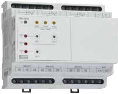
The hot spot 3 relay accepts up to three inputs from resistance temperature detectors (RTD) and provides up to three user adjustable trip points which can be used to initiate alarms, cooling system or shutdown. The relay is ideally suited for the protection of electric motor windings, transformers, generator winding and bearing temperature. The analogue output can be used for remote monitoring of high temperatures.
