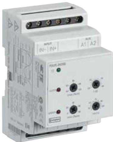
The DC volts, millivolts and transducer trip relay protectors provide continuous surveillance of DC voltages or current signals. When the input signals move outside the set point limits the relay will operate and the fault LED will illuminate.
