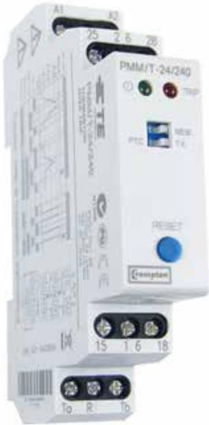
The Thermistor protector trip relay monitors the temperature of a motor using the PTC sensor (positive temperature coefficient resistor) or thermostat (TK) switch built in to the motor winding. Relay contacts can be used to disconnect the supply to the motor should it overheat. LEDs indicate mains on and fault status.
