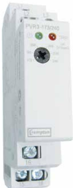
The phase sequence and phase failure protector trip relay is designed to monitor the correct phase rotation or sequence of a three-phase supply system. It provides protection against incorrect phase sequence, loss of one phase and under voltage. Two versions are available to suit either three-phase three-wire (PVR3) or three-phase four-wire (PVR4) systems.
