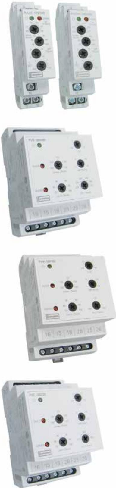
When the measured voltages moves outside the set point limit for longer than the time delay, the relay will operate giving an alarm control or tripping signal. The Protector can be used for under and over voltage detection, start standby generators, operation of mains failure units and switching standby suppliers. An illuminated red LED indicates a fault condition. The three-phase, three or four-wire models with protect each phase independently.
